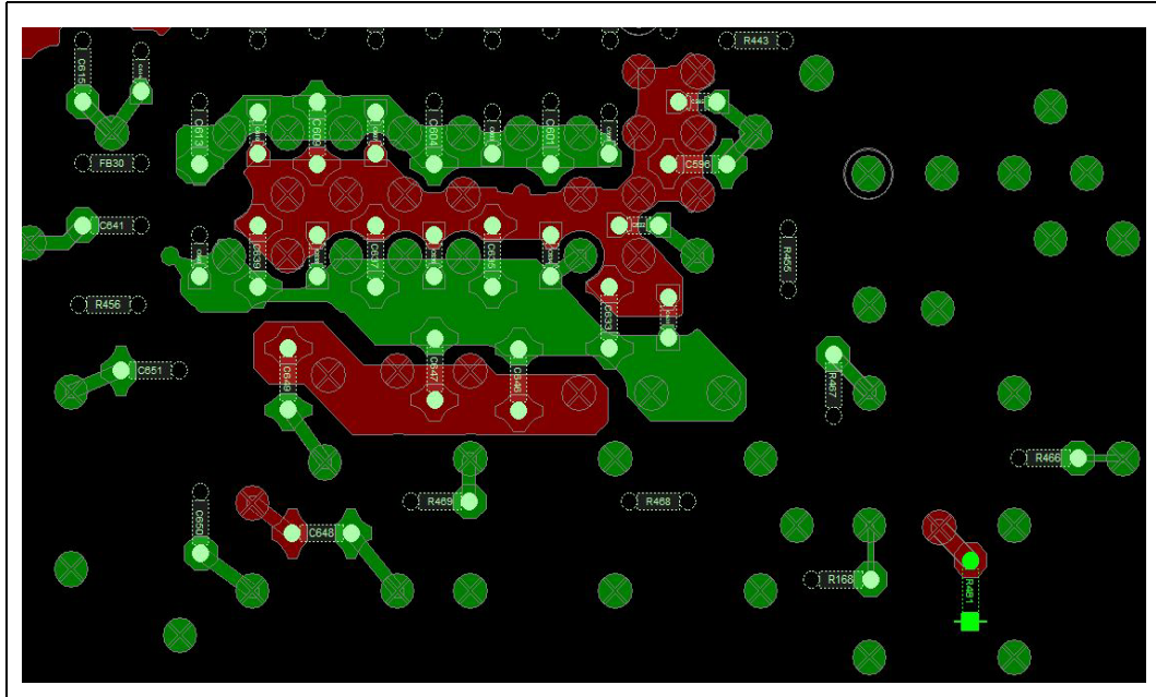
Figure 15-28. V1P05 VR VSense - Sense Across R481
