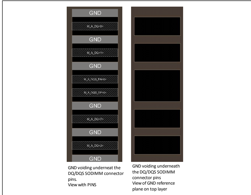
Figure 4-22. SODIMM DQ/DQS Pad Void
