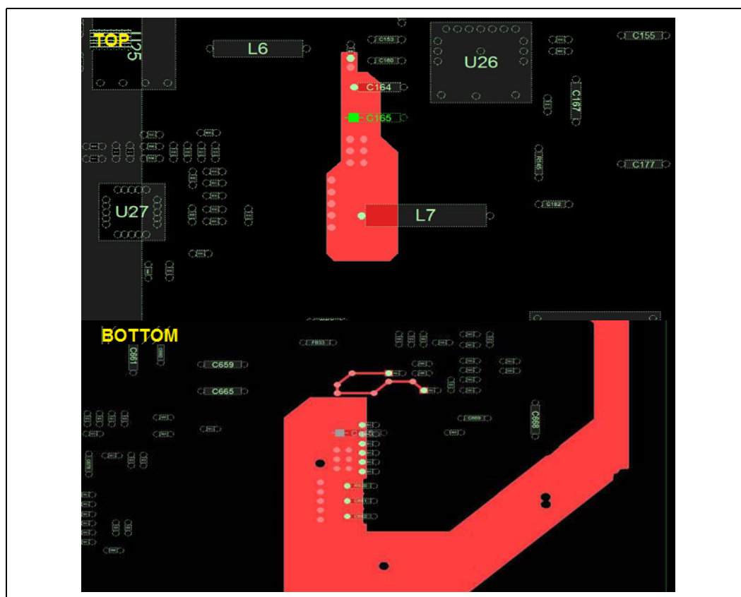
Figure 15-30. V3P3 Decoupling Capacitors
