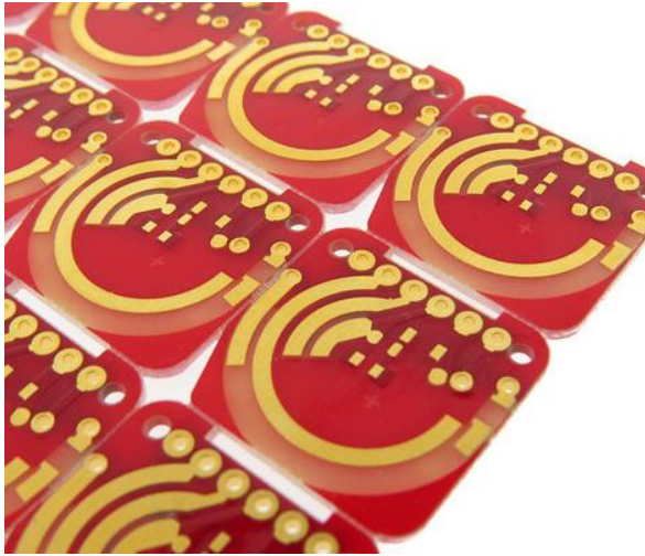
Figure 13: Example of a Full Body Hard Gold Surface Finish
