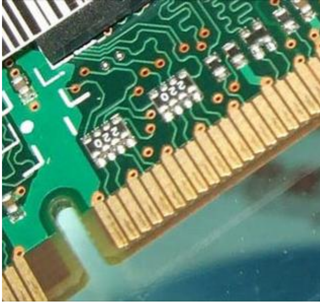
Figure 14: Example of Edge Connector Plating
