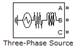
Figure 11.46. The SimPowerSystems Three-Phase Source block
