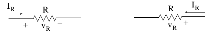
Figure 2.2. Voltage polarity and current direction in accordance with the passive sign convention
