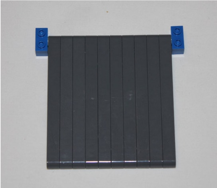
Figure 1-30. The Technic bricks are added to the beams via the frictionless pins
