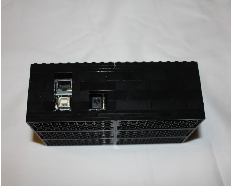
Figure 3-13. The back of the box shows how the Ethernet, USB, and power ports are easily accessible
