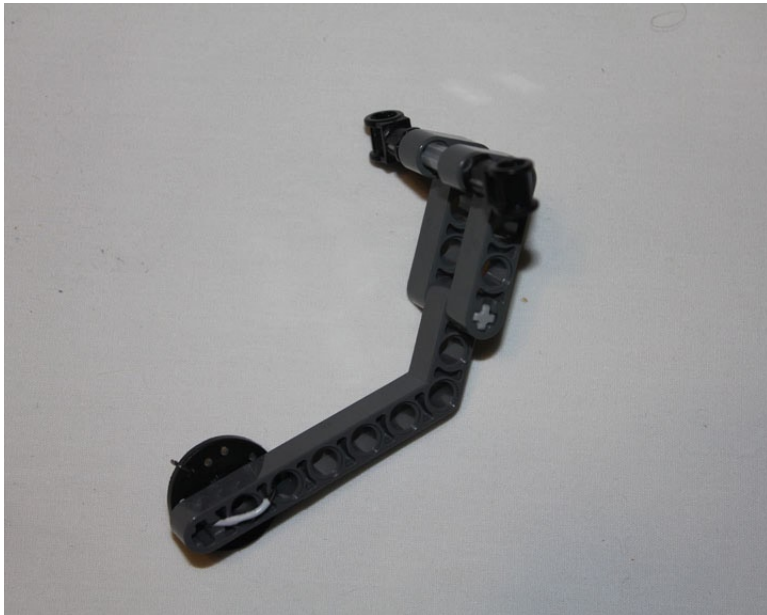
Figure 1-22. Angled Technic beams are added to the end of the secured Technic beam, and a 5M pin and two angle connectors hold it in place
