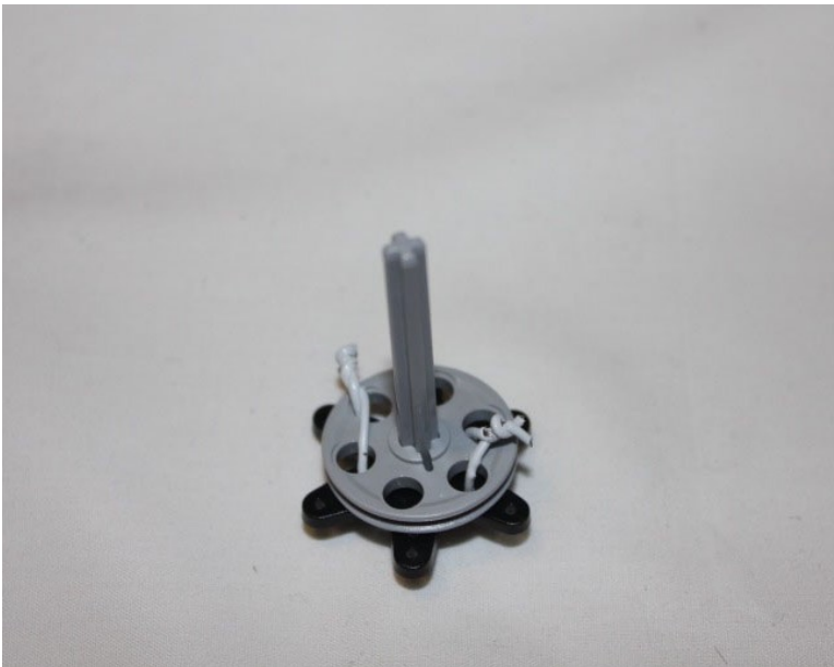
Figure 2-37. The wheel and the servo motor attachment are wired together and the 5M pin is inserted into the hole
