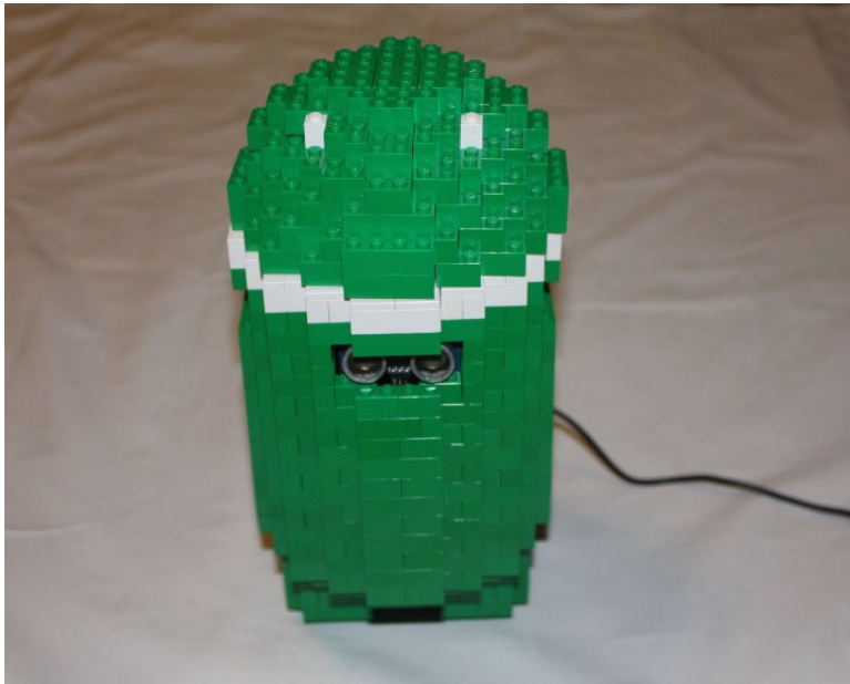
Figure 2-46. The Android stands on its new legs. The outer edge of the legs should line up with the outer edge of the lowest level of the Android's body
