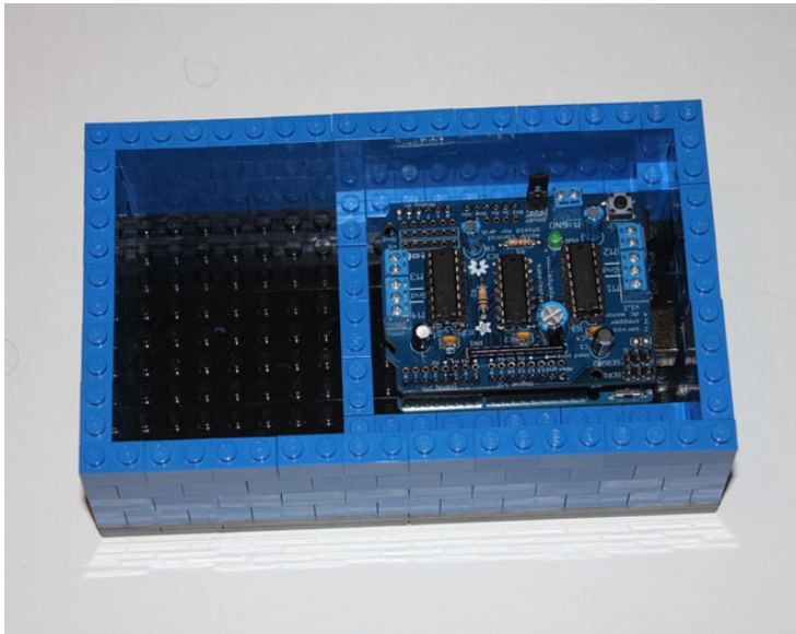
Figure 1-18. The Arduino is easily seated into the section you made for it
