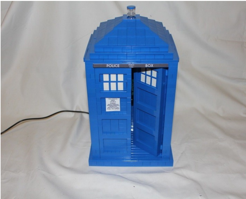
Figure 5-46. The LED is attached to the ground and pin 6, the lid is placed onto the top of the body, and the TARDIS is completed
