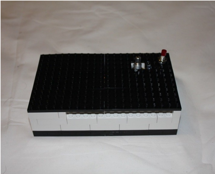
Figure 6-6. The first layer of the lid is laid down
