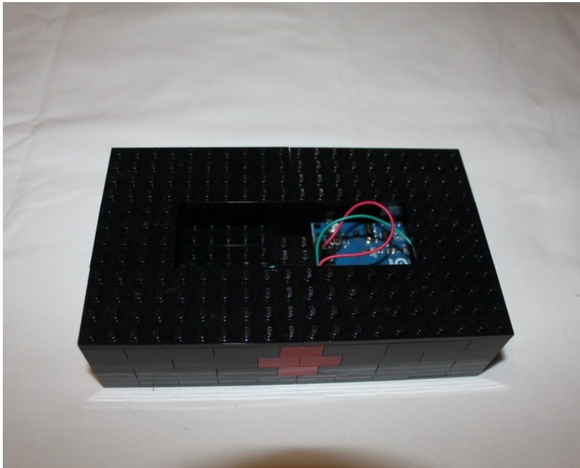
Figure 4-8. The first layer of the lid leaves a wide hole that does not secure the column behind the RFID reader
