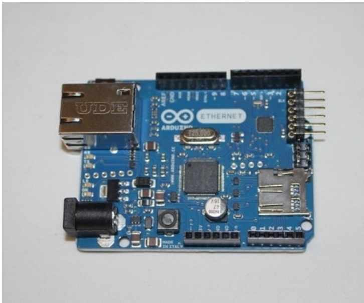
Figure 3-1. The Ethernet Arduino. The port on the top left is an Ethernet port rather than USB
