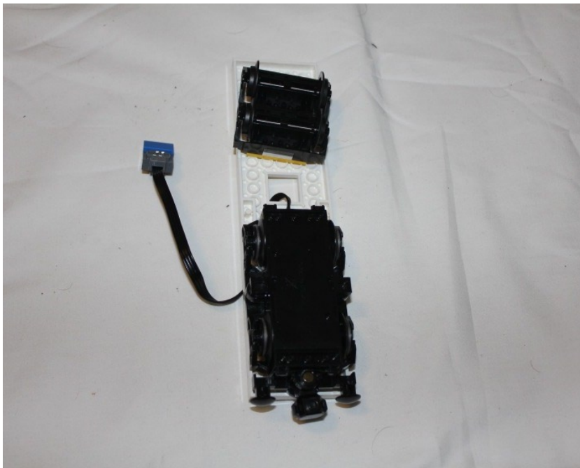
Figure 6-12. The wheels are connected to the bottom and the cable from the back wheels is pushed through a hole
