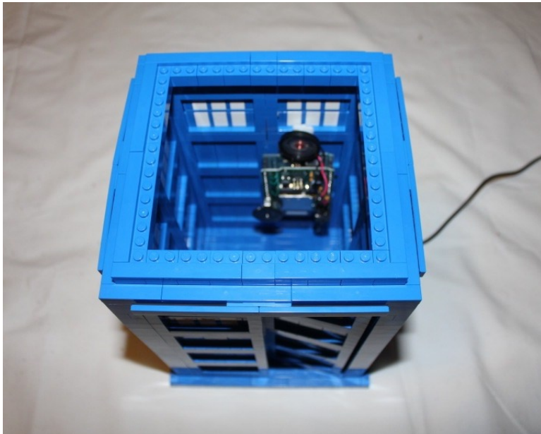
Figure 5-33. With the additional 2 \times 2 bricks placed around the top of the TARDIS, tiles are to be placed around the edge
