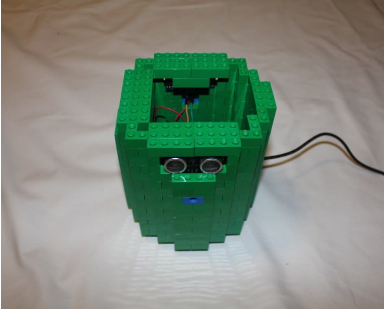
Figure 2-24. The layer above the ultrasonic sensors covers them
