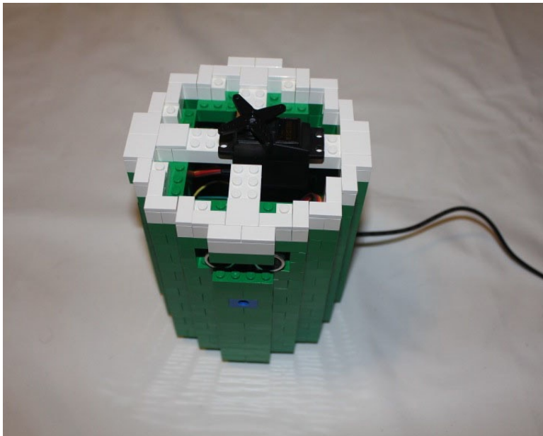
Figure 2-26. A layer of tiles is added to allow smooth movement of the head and to support the servo motor
