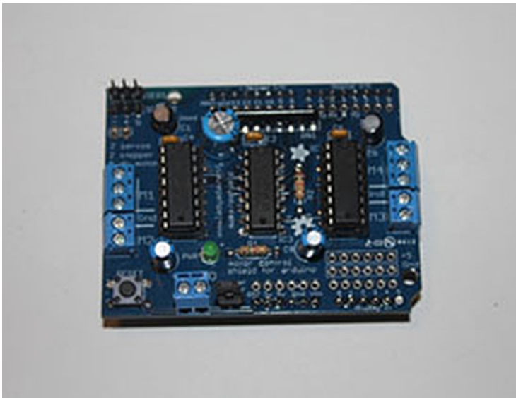
Figure 1-6. The assembled motor shield
