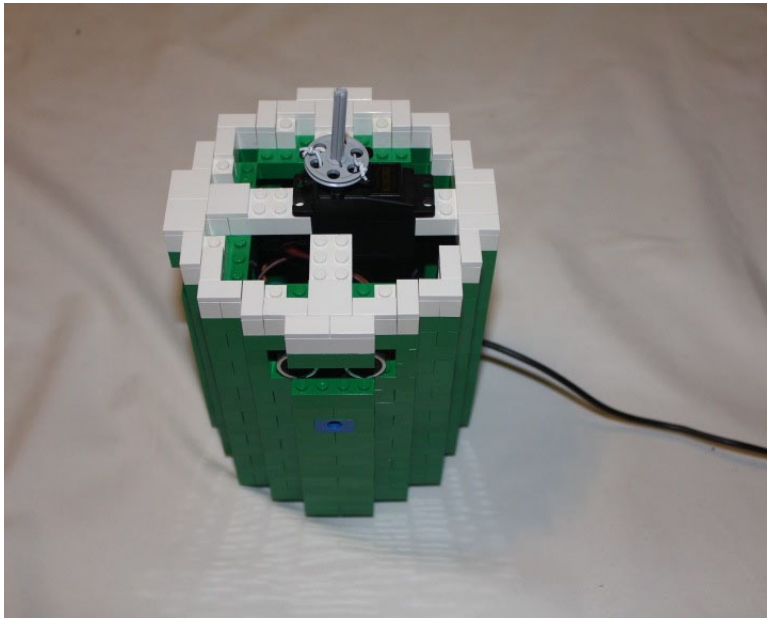
Figure 2-38. The attachment is put on the motor. Check which direction the motor is pointing to know which direction the head will face
