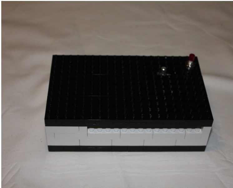
Figure 6-8. The lid is completed, exposing the potentiometer, button, and IR LED in the back corner
