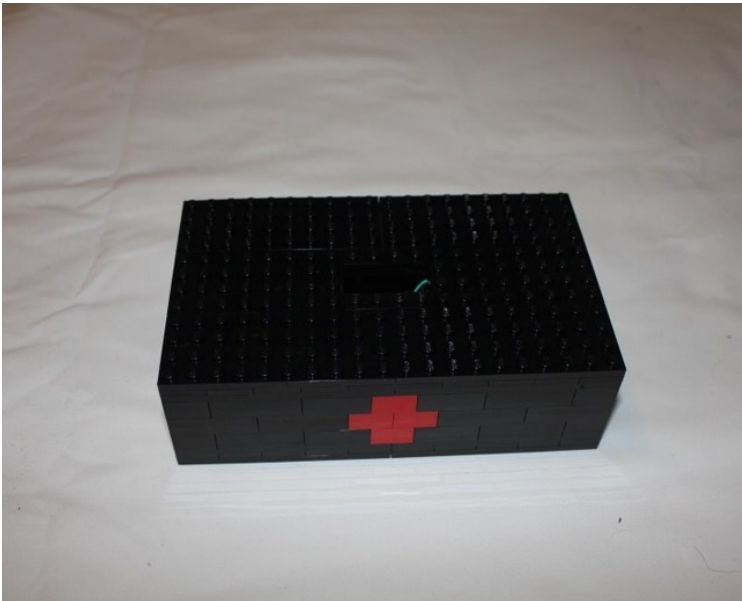
Figure 4-10. The third layer of the lid secures it in place while leaving a hole in the middle for wires
