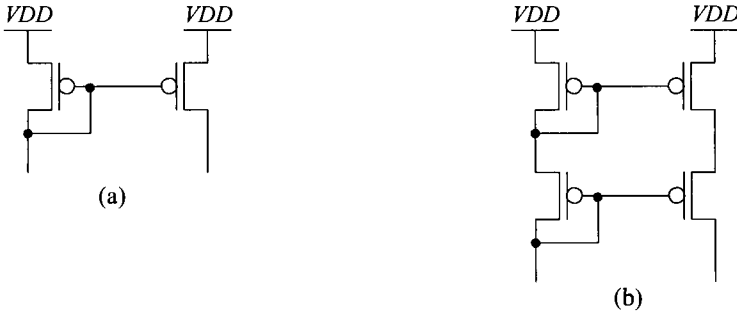
Figure 23.8 Using a current mirror to force the same current through each side of a reference.
