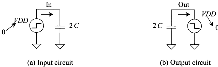
Figure 10.3 Splitting the capacitor in Fig. 10.2 up into two equivalent capacitors for developing a model.
